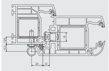
**Load capacity with 2 hinges** 80 kg
