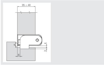
**Load capacity with 1 pair** 80 kg
